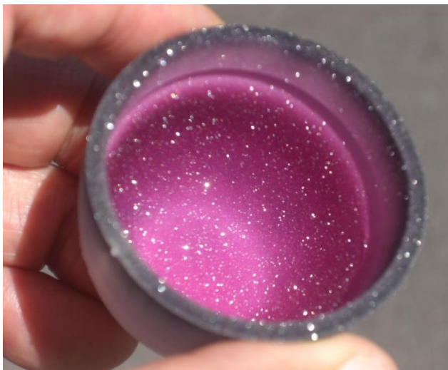
図4 太陽光下のルビーコーティングるつぼ (Fig.4 Photograph showing the ruby-coating crucible viewed under sunrays)
