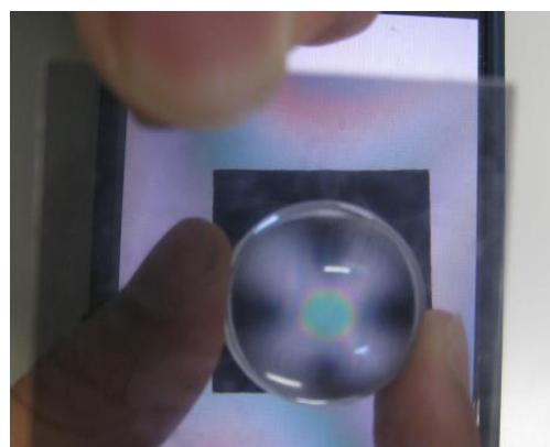
図4 水晶玉の異方性観察 Fig. 4 Observation of anisotropy in a crystal ball
